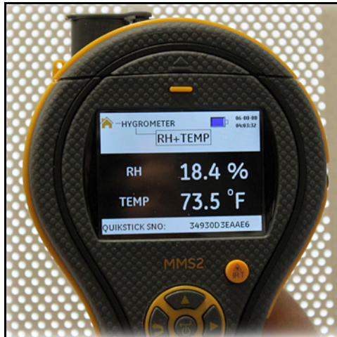
Figure 4: MMS2 as a Hygrometer
