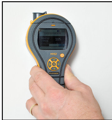
Figure 3: Taking Relative Moisture Readings
